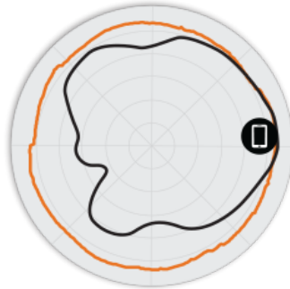
Figure 3. 5GHz Azimuth Antenna Patterns
