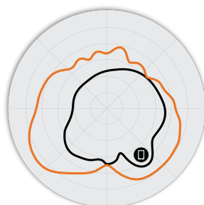
Figure 3. R350 5GHz Azimuth Antenna Patterns
